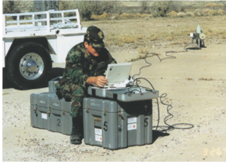
Figure 2.7: A system PINS (Portable Isotopic Neutron Spectroscopy) for identification of munition and chemical weapons used by US army [88].
