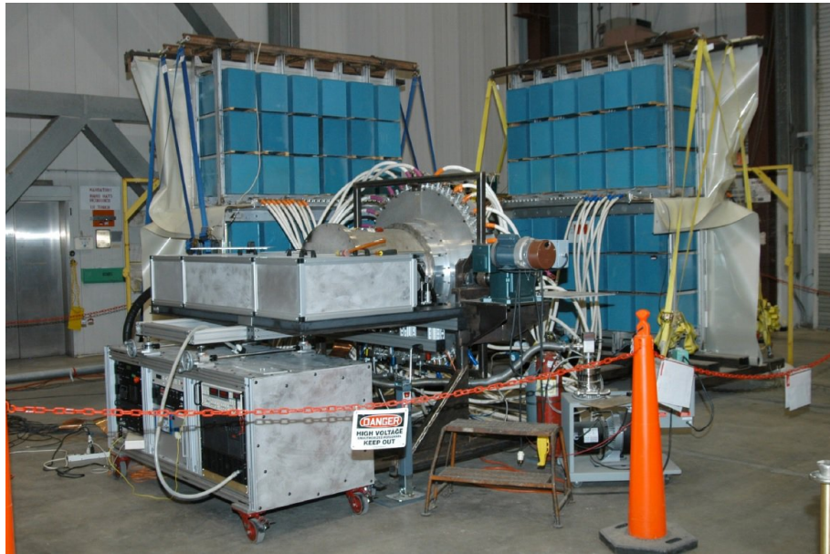
Figure 2.9: The Gemini plasma focus: stored electrical energy of 1 MJ, current pulse maximum of 3 MA, DD neutron yield above 10^{12} per single shot [57].
