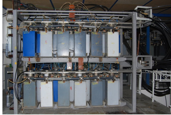
Figure 3.1: One of the 12 modules of the capacitor bank of the PF-1000 pulsed power generator.
